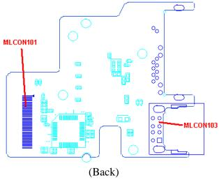
Figure B-3 LAN Board layout (front/back)
